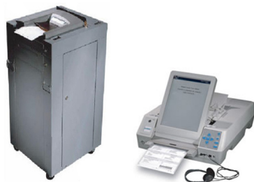
Above: One optical scanner and one ballot marking machine to assist voters with disabilities or language barriers replaces about 10 touch-screen voting machines (below).
